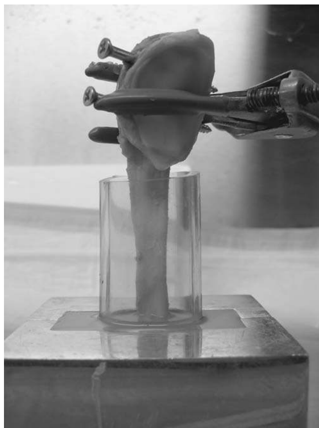
Figure 2. The patella and tibial tubercle were potted with the base of the plastic tubing forming a sealed container around the tendon. This tubing was filled with artificial synovial fluid to immerse the tendon for the remainder of the experiment. In this way, desiccation of the tendon was prevented during extended testing times.
